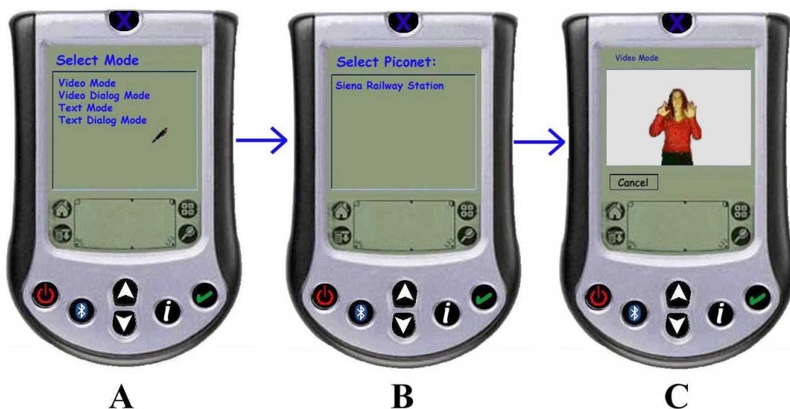
Figure 12: Client operation. A: configuring the preferred output mode. B: selection of the Blue Sign Piconet. C: playback of the video in Sign Language
