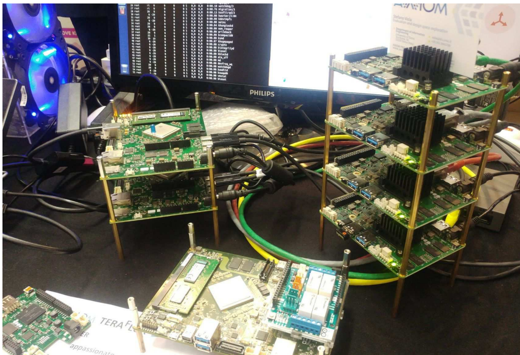
Figure 11. A cluster of AXIOM boards and UD00 X86. Presented on the UD00 booth.
