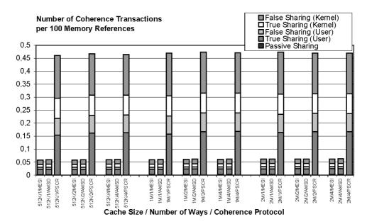
**Figure 4** Number of coherence transactions vs. cache size (512K, 1M, 2M bytes), number of ways (1, 2, 4), and coherence protocol (AMSD, MESI, PSCR). Coherence transactions are invalidate transactions in MESI, and AMSD, write transactions in PSCR. Data assume four processors, 64-byte block size, and an affinity scheduler
