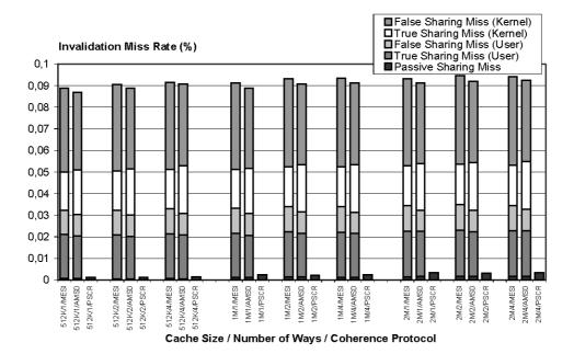
Figure 3 Breakdown of miss rate vs. cache size (512K, 1M, 2M bytes), number of ways (1, 2, 4), and coherence protocol (AMSD, MESI, PSCR). Data assume four processors, affinity scheduling, and 64-byte block
