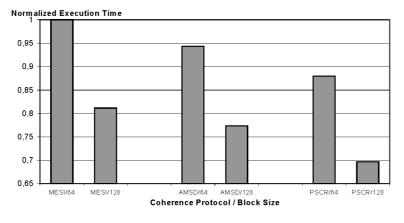
Figure 9 Normalised execution time vs. block size (64, 128 bytes) and coherence protocol (AMSD, MESI, PSCR). Data assume, an affinity scheduler, 1M-byte 2-way set associative caches. Execution Times are normalised with respect to the execution time of the MESI, 64 byte block configuration
