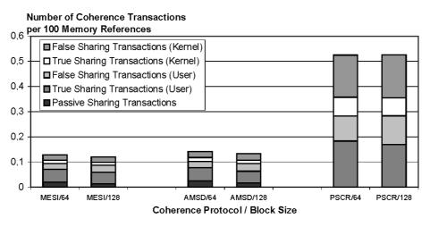
Figure 12 Number of coherence transactions vs. coherence protocol (AMSD, MESI, PSCR) and block size (64, 128 byte). Data assume an affinity scheduler, 1M-byte 2-way set associative caches
