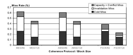
Figure 10 Breakdown of miss rate vs. coherence protocol (AMSD, MESI, PSCR) and block size (64 byte, 128 byte). Data assume an affinity scheduler, 1M-byte 2-way set associative caches. There is a decrease of Cold, Capacity+Conflict miss components, and a little decrease of invalidation miss component
