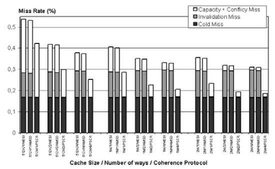
**Figure 2** Breakdown of miss rate vs. cache size (512K, 1M, 2M bytes), number of ways (1, 2, 4) and coherence protocol (AMSD, MESI, PSCR). Data assumes four processors, affinity scheduling and 64-byte block
