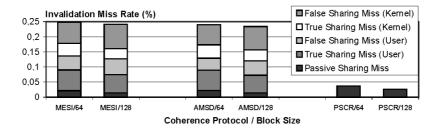
Figure 11 Breakdown of invalidation miss rate vs. coherence protocol (AMSD, MESI, PSCR) and block size (64 byte, 128 byte). Data assume an affinity scheduler, 1M-byte 2-way set associative caches. Passive Sharing Misses decrease when increasing block size because the invalidation unit is larger
