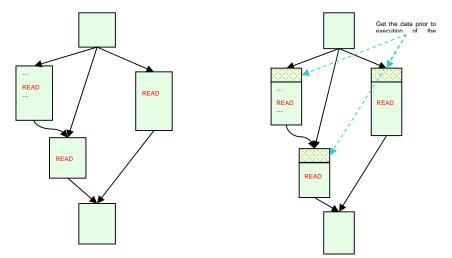
*Figure 3*. Mechanism for pre-loading data. On the left, current generic situation is shown (arrows represent the data being communicated). On the right, preload phase has been added to each thread that will include all memory accesses within the thread.
