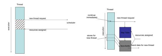
Figure 2. Blocking (on the left) and non blocking resource assignment (on the right)
