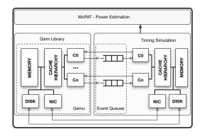
Figure 1: The proposed kilo-core simulation framework
