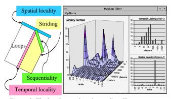
Figure 3. The locality surface for median filter program.
