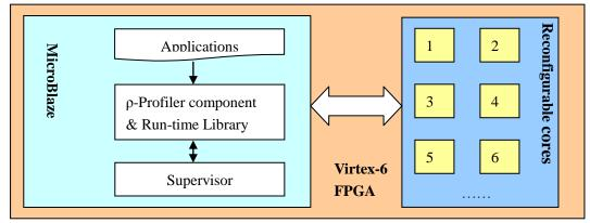
Figure 1 Overview of the reconfiguration framework
