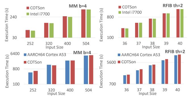
Figure 1: Performance validation of the benchmarks Recursive Fibonacci (RFIB) with 2 as threshold (th) and Matrix Multiply with 4 as block size (b) between the COTSon simulator, the Intel i7700 (top) and the ARM Cortex A53 (bottom) architectures.
